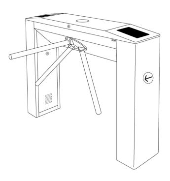
Anti-tailgating. Smart lock mechanism uses proximity switch to detect rotation and effectively relock back after 1 person pass through. Also support time delay 5 sec, 10 sec, 15 sec and 60 sec.
