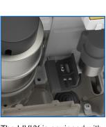
The LIVI/X is equipped with a new magnetic limit switch system, consisting of a new technology sensor and a set of magnets attached to the multi-adjustable rack.
